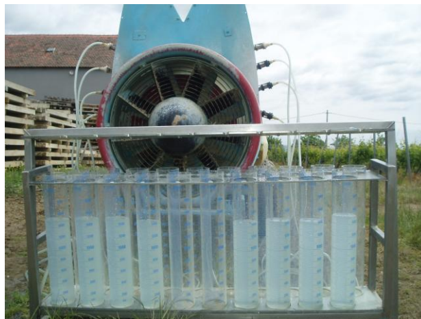
Figure 5. The device Volos II for measuring nozzle flow on mistblower
