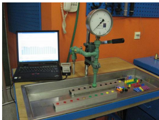
Figure 4. Desktop - electronic device for measuring nozzle flow
